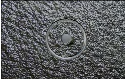
Figure 15. Scored TriArmor® Corrosion Protection System
